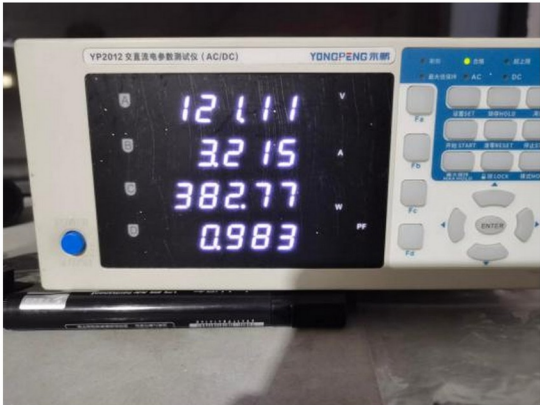
Electrical input measurement.
