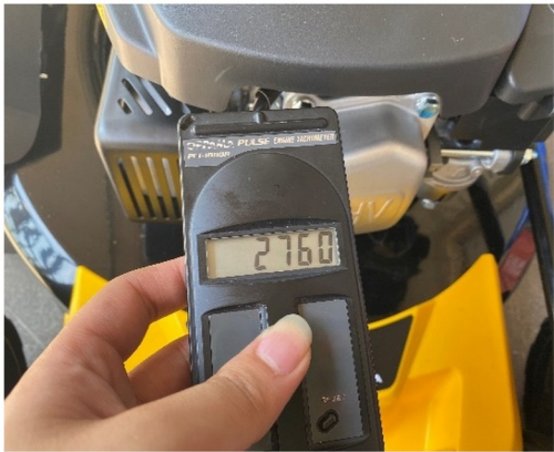
No-load speed measurement: 2,760 r/min.
