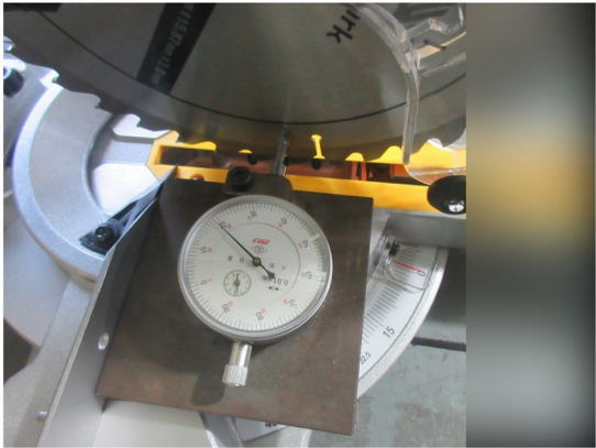
Representative alignment measurement; blade identity obscured.
