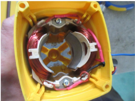
Stator and winding inspection.
